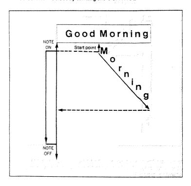
As shown by the diagram, when the start point is set to the beginning of "M", "Morning" is played back when a key is pressed. By adjusting the start point in this way, it is possible to start playback at the necessary portion.
