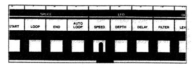
Press the LFO SPEED button on the front panel. The LCD will read:
