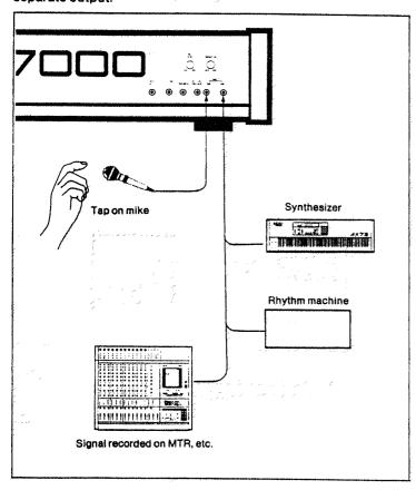
To perform playback using auto trigger, connect the trigger source to the MIC or LINE input jack on the rear panel. Now press the AUDIO TRIGG button.
