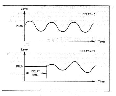
/ith the LFO vibrato effect, different parameters can be set for ach voice when performing multiple point sampling. The effect an also be applied by operating the modulation wheel.
