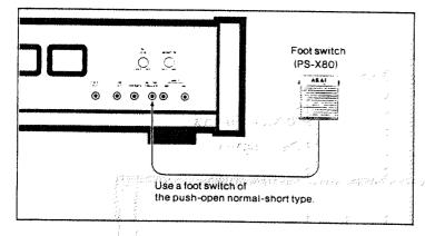
For sampling, use exactly the same procedure as for basic sampling, multiple point sampling, or overdubbing. Once preparations for sampling are completed, prepare the input source, then press the foot switch to start sampling (or overdubbing).
