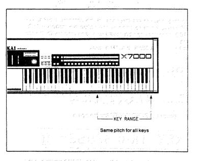
This function is handy for percussion sound effects in which differences in pitch are not desired.
