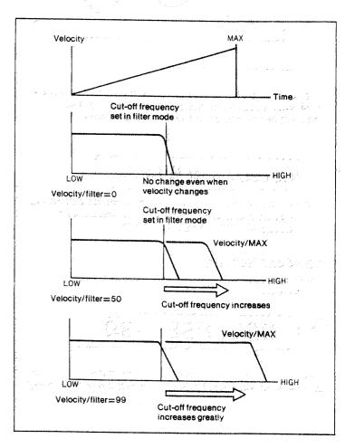
When instruments are played loudly, the harmonics can be heard clearly, resulting in a bright sound. This phenomenon can be recreated on the X7000 using the velocity/filter setting mode. Use it for piano, strings, brass, or percussion instrument voices. These are the basic ways of editing the sampled sound. Transposing and tuning are explained in the Programming section which follows.
