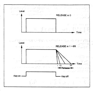
Turn the CONTROL knob to change the value between 0 and 99. The higher the value, the longer the release time. The sustain/resease effect is also possible by receiving sustain pedal data.
