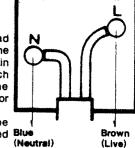
Do not connect any wire to the larger pin marked E or \(\pm\) when wiring a plug. Ensure that all terminals are securely tightened and that no loose strands of wire exist.
