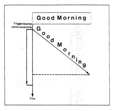
If the trigger source sound is longer than the recording time of the sampled voice data, the "Good Morning" will be played back completely. For a very short trigger source sound, only a short "G" will be played.
