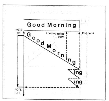
When the looping splice point is set as shown in the diagram, the portion between the looping splice point and the end point will be played back repeatedly.
