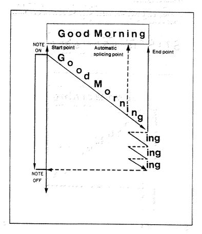
When the looping mode is set, the automatic splicing system is automatically called out and the optimum splicing point is found near the end point to produce continuous sound. The looping mode is perfect for playing strings, brass, or a chorus. If the CONTROL knob is turned clockwise further, the LCD will switch to the alternating mode.
