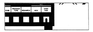
The LCD will now be in the basic pitch setting mode. Use the CONTROL knob to set the basic pitch of the next sound to be overdubbed, then press the OVER DUB button.
