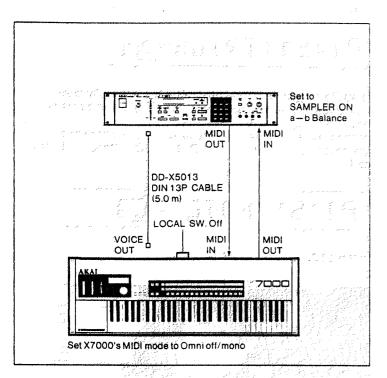
Use the separately sold Akai DD-X5013 13-pin DIN connector cable to connect to the synthesizer.
