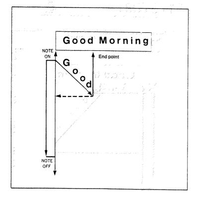
As shown by the diagram, when the end point is set before "Morning", only "Good" is played back when a key is pressed, "Morning" being cut.
