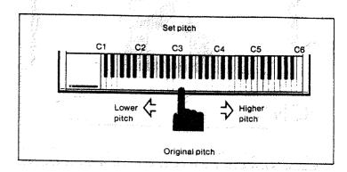
This is the basic procedure for sampling on the X7000. Now let's see how multiple point sampling, one of the outstanding features of the X7000's works.
