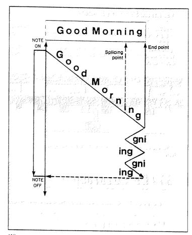
When set as shown in the diagram, the sound "Good Morning" is played once, "gni" then "ing" will be replayed continually between the splicing point and end point until the key is turned off.
